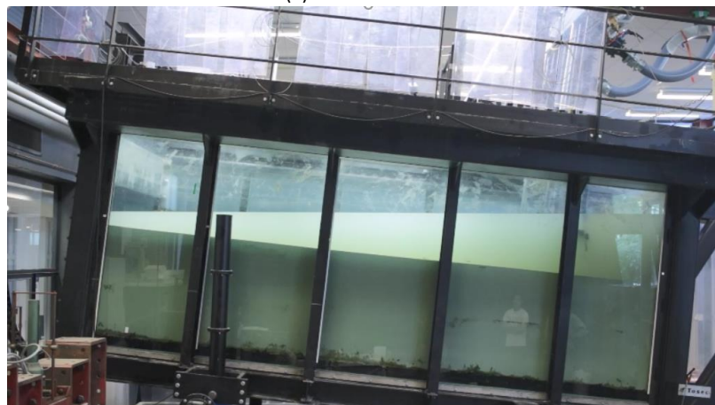
(b) Tilted liquefaction tank and stable seabed
