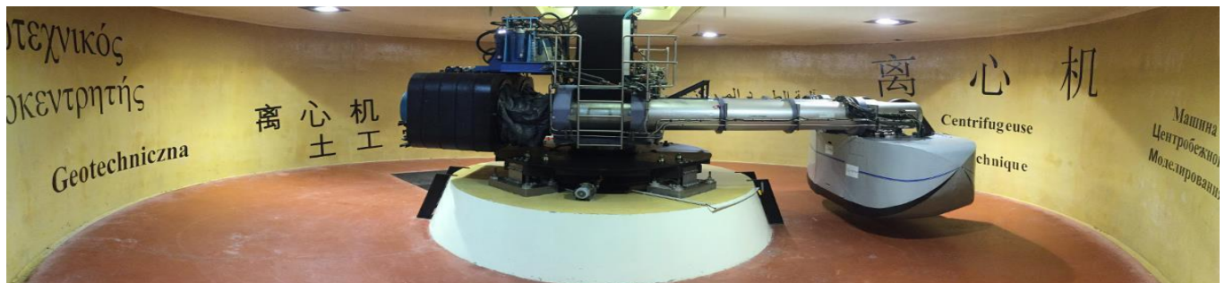
Figure 44 The 200xg-ton Centrif-UGE (5.5m radius)
