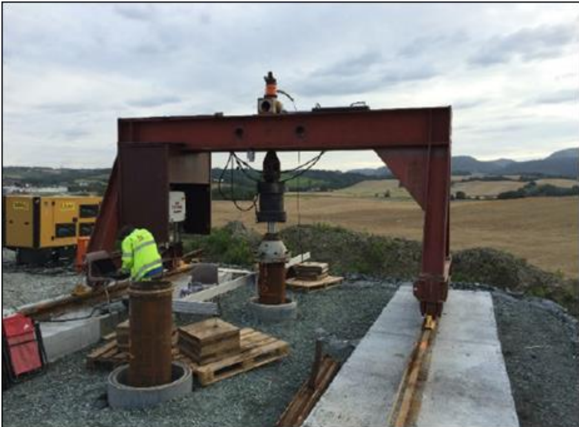
Figure 90 Full-scale testing of pile capacity in a geo-test site
