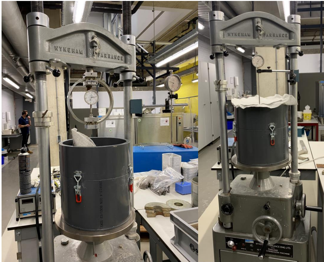
Figure 25 Clay consolidation system of the geotechnical centrifuge of TU Delft
