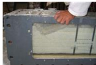
Figure 49 Preparation of a test of wetting-induced collapse in embankment base
