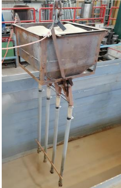
Figure 77 The Dry Pluviation System consisting of a sand hopper and four rigid tubes
