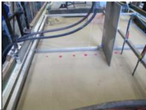
3. The sheet pile wall (I 90 w 60 x d 1 cm) was vibrated into the sand package in the center of the model container for a few minutes at a speed of 3 mm / s (30 Hz).
