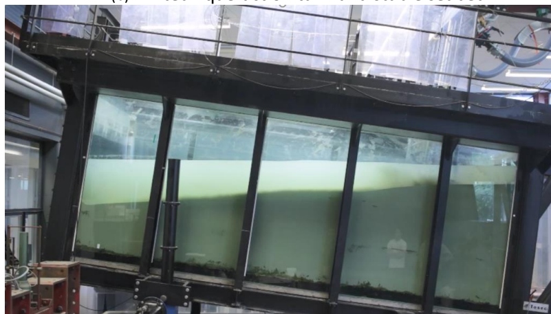
(c) Tilted liquefaction tank and liquefied seabed
