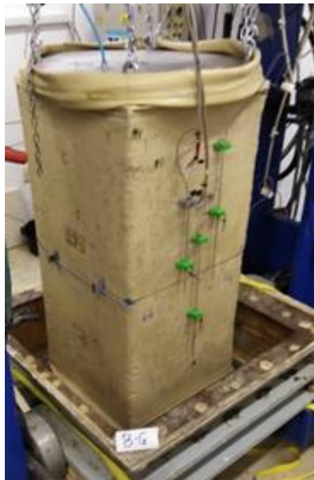
Figure 8 Prismatic specimen for triaxial test. Local LVDTs attached on side.
