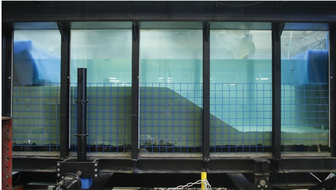
Figure 40. Submersed slope in the Liquefaction Tank prepared with the suction dredging system and the shallow waves absorbers
