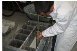
Figure 49 Preparation of a test of wetting-induced collapse in embankment base
