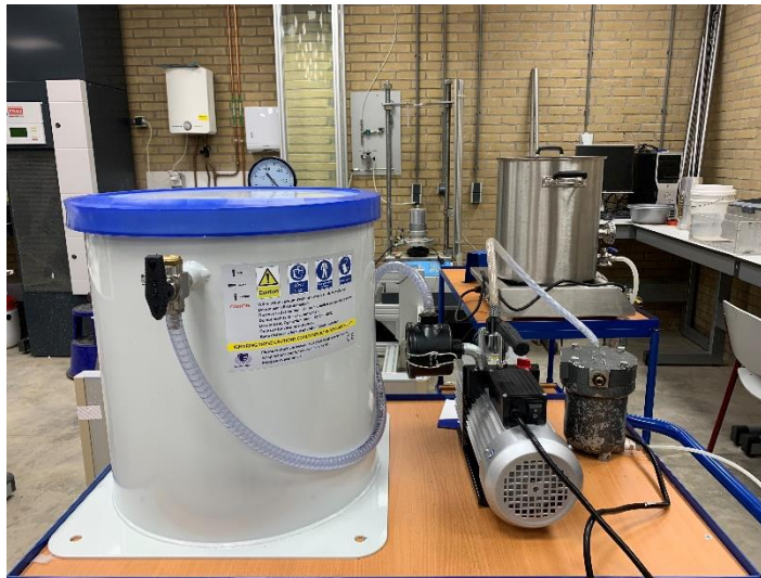
Figure 24 Vacuum chamber of the geotechnical centrifuge of TU Delft
