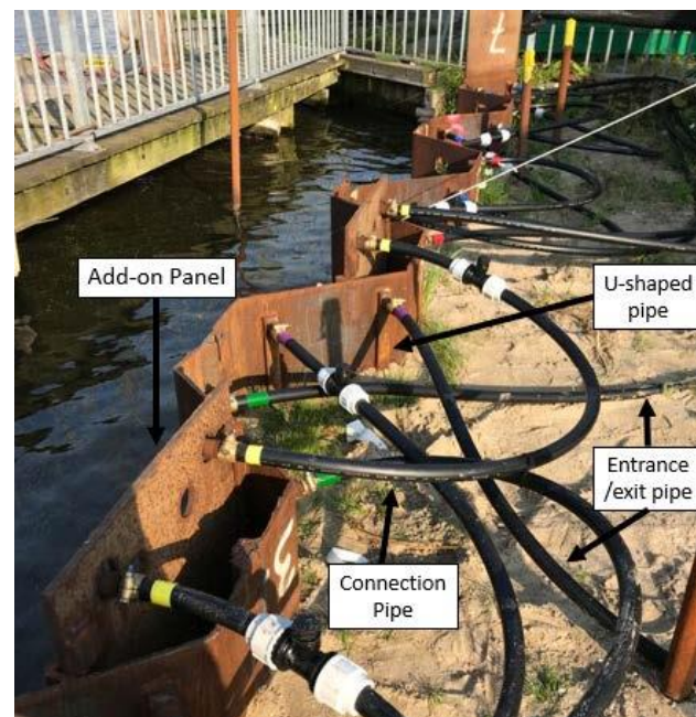
Figure 2. a) UniMI thermo-mechanical apparatus, b) Energy quay wall test site installed in The Netherlands (Gerola et al., 2025)
